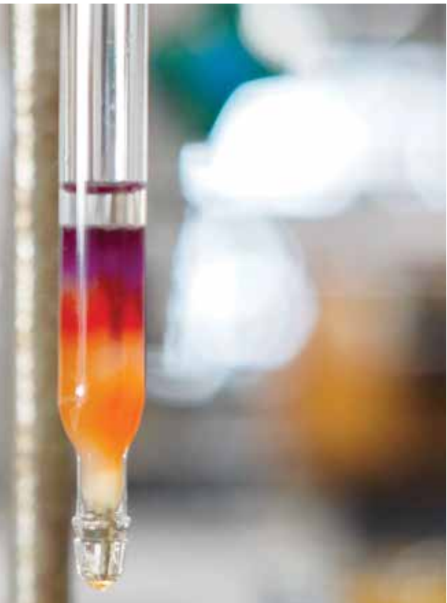
Separate color by column chromatography
