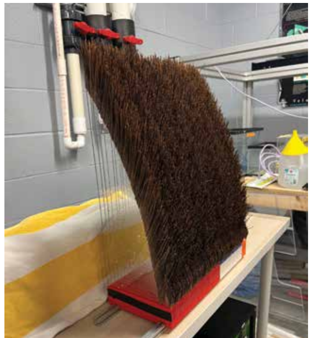
A model of acrylic and palm tree wood fiber used to investigate how baleen plates in a humpback whale's mouth filter out microplastics
